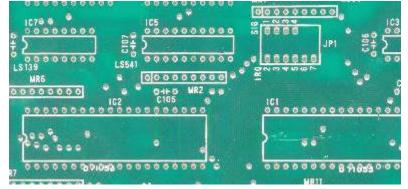
The panels are coated with flux – a viscous compound that promotes even coating of the copper. Then the panels are dipped completely into a bath of molten solder. The solder covers all exposed metal surfaces. As the panel is removed from the solder, high pressure hot air is directed at both sides of the panel. The "blast" of air removes excess solder from the holes and smoothes the surface of the pads.
