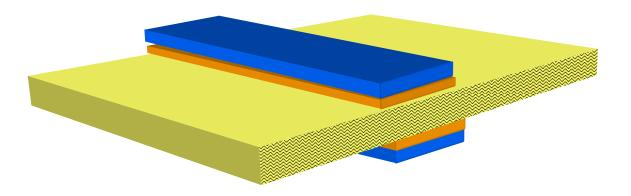
Then the copper is chemically removed from the core in all areas not covered by the dry-film resist. This creates the copper pattern that matches the film pattern. The core laminate surface is exposed in areas where copper was etched away.
