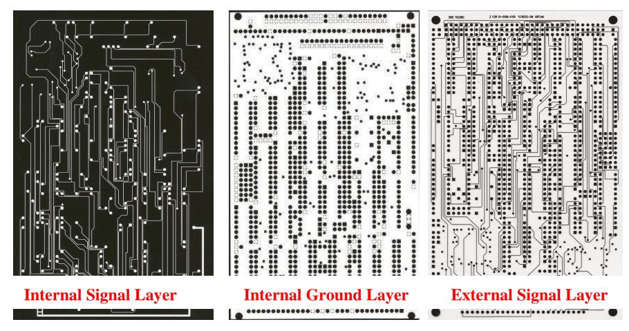
Each of the circuit and land patterns are unique to that part number and each layer has its own artwork pattern or piece of film. Inner layer film is negative and outer layer film is positive.
