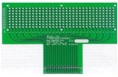
Then the boards are generally checked for cleanliness, sharp edges, burrs and other fabrication requirements. Chamfers, slots, countersinks and bevels are added during the rout & fabrication processes.
