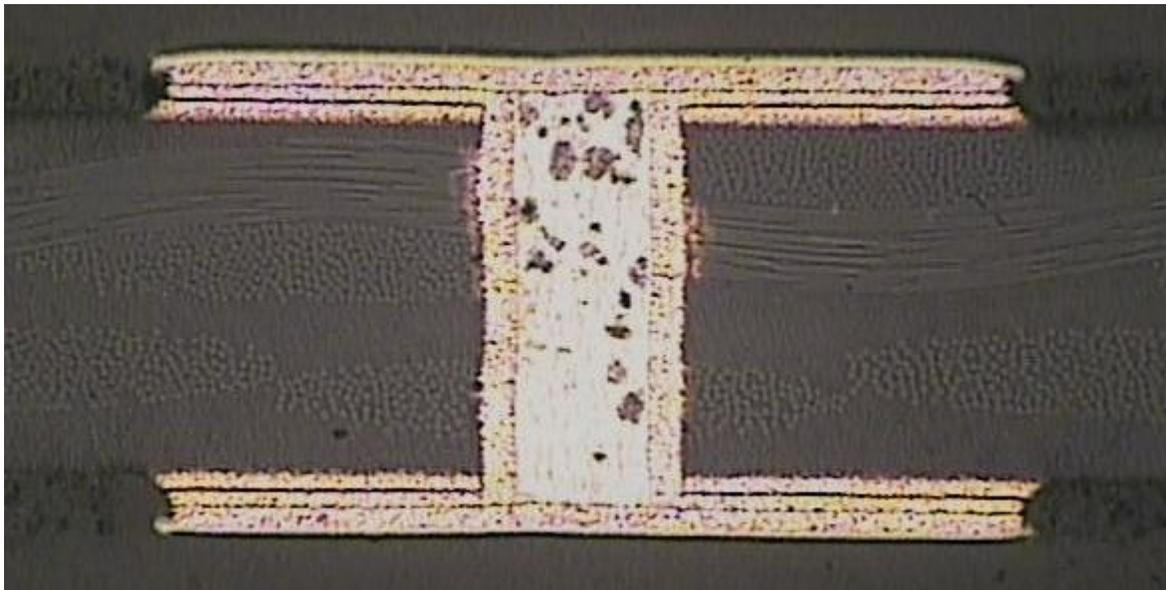
Figure 1 - Dupont CB100 Conductive Via Fill
