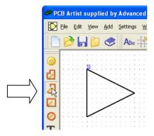
Select a start point 100 mils down from the symbol origin 'S' on the vertical segment (2 grid points), drag a line 100 mils (2 grid points) to the left. Like this:
