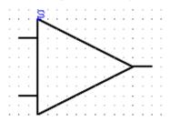
Position the two additional lines as shown above. At this stage PCB Artist does not recognize these lines as electrical connect points or pins, we are now going to insert these.
