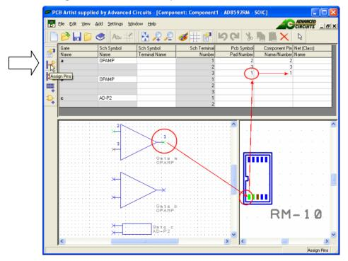
Click on the **Assign Pins** button on the Component toolbar.
