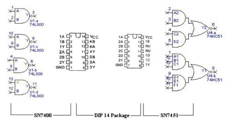
The 14-pin DIP (Dual Inline Package) is used on 1,000s of different components. For efficiency, we only want to store the 14-pin DIP PCB footprint once and then use it repeatedly to build different Parts or components that specify a 14-pin DIP footprint.
