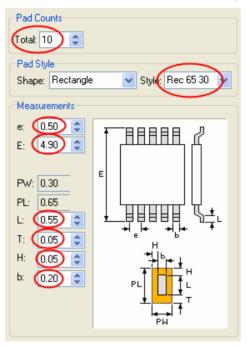
In Measurements, you need to enter the dimensions to be used. Generally speaking, these will be located on the manufacturer's datasheet or in another central resource, such as the IPC Council standard.
