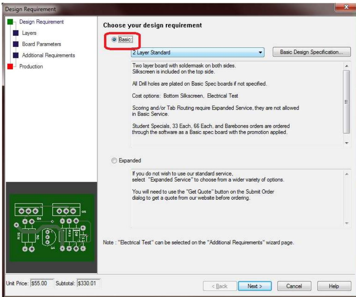
The PCB Configuration is also where one can set up the board order. Make sure your order matches the 33Each or 66Each specs found here: <https://www.4pcb.com/pcb-prototype-2-4-layer-boards-specials.html>
